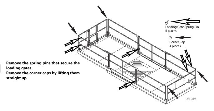
Slide the loading gates away from the load area, then pivot away from the guard rails. Lay the gates in the front section of the platform.
