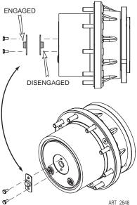
Disengage Brakes before Towing or Winching
