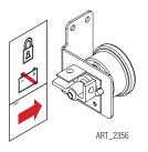
• Check Battery Disconnect Switch outside the front end of the Engine Module. Must be in ON position.
